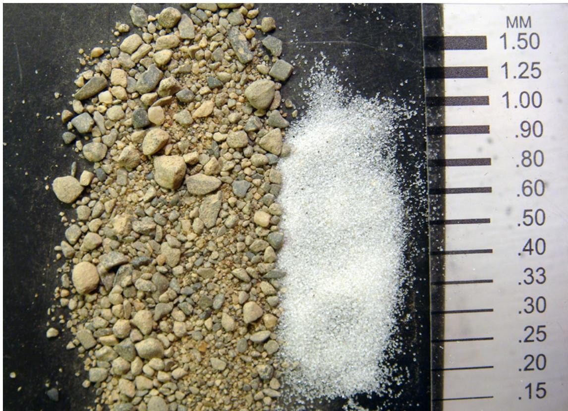
Figure 1: Fine quartz sand used in PHLc grout at right; a conventional masonry sand at left
